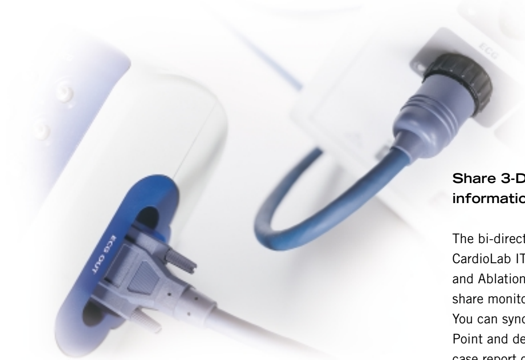
12-lead ECG Quick Connect cable between GE's CardioLab and Biosense Webster's CARTO XP System.
